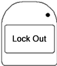
A fail will be followed by a “**Lock Out**” message on the display followed by the BAC reading recorded. The vehicle cannot be started and the driver will be prevented from attempting another test for at least **5** minutes (countdown will appear on the LCD screen).
