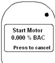
**Important:** Attempting to turn the ignition on in the vehicle prior to the “**Start Motor**” message appearing will result in “**Key off**” message.
