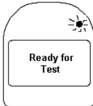
Wait for the Handset to display **“Ready for Test”** and the status light to change to flashing green. The wait time will vary depending on the ambient temperature (this may take up to 3 minutes, particularly in cold weather).
