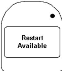
Attempt to start the vehicle by using the ignition key. If the unit is in stall protect, it will restart without a test.
