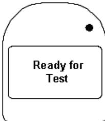
If “**Ready for Test**” is displayed, you need to pass a breath test to start the vehicle.
