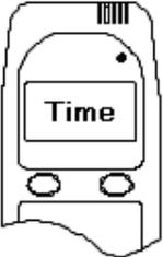
A line drawing of a mobile handset. The screen displays the word "Time" in a rectangular box. Above the screen is a speaker grille and a small circular indicator light. Below the screen are two circular buttons.                                         | <p>Press and hold the left button to access the user menu.</p> <p>Use the left button to scroll to <b>"Time"</b>.</p> <p>Press the right button to select this option.</p>                                         |
